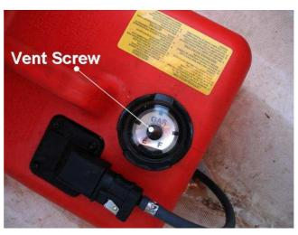
it, you may hear air rushing in or out; it's good to have a vent system that works on the tank! Close the vent at the end of the day when you hose the launch down. If you don't open the vent the engine will only run for a limited amount of time before the vacuum takes over and starves the fuel system giving you a nice paddle out of harms way from the middle of the river should you forget; it's most likely you'll only do this trick once.
