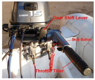
will only damage the engine if attempted. The Tiller Throttle Control and Gear Shift Lever Systems must be kept lubricated as part of this engines general maintenance or the remote system will not work.
